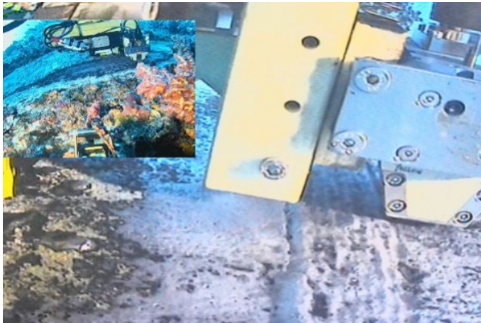
MagCrawler performing ACFM inspection
