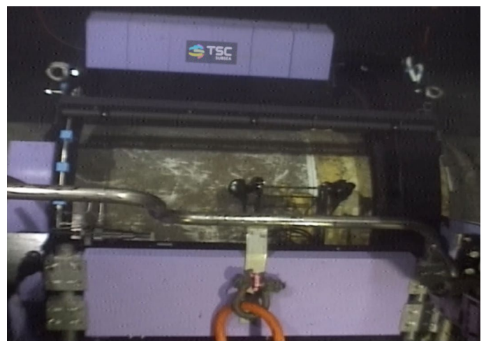
ARTEMIS® Performing Full 360° Circumferential Inspection
