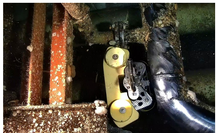
LineScanner examining a bend with restricted access
