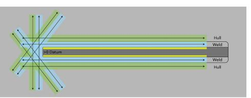
Thanks to the consistent and controlled scan speed throughout the inspection, the scans exhibited a high signal-to-noise ratio, instilling confidence in the inspection results. This ensured that the reporting threshold for a surface-breaking defect of 20 mm in length x 2 mm in depth and larger could be easily detected throughout the inspection campaign.
