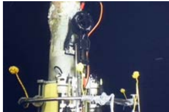
Phased array complex weld inspection
