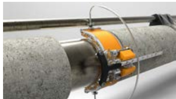
Pipeline 360-degree scanning
