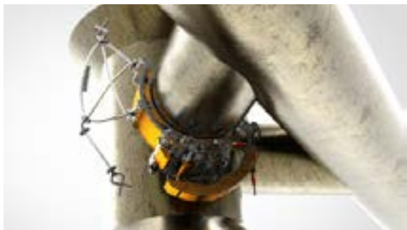
Tight access 3-axis scanning
