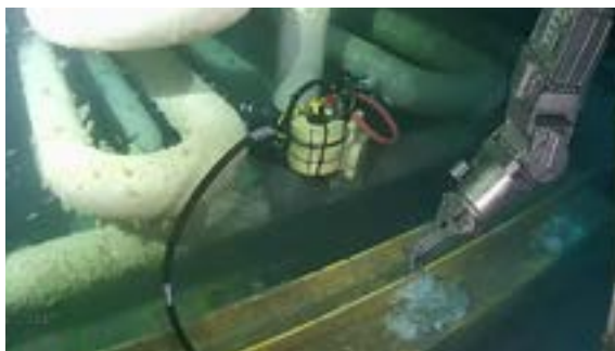
Limited access motorised scanner
