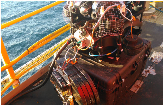
Figure 1: ACFM® MagCrawler™ on deck
