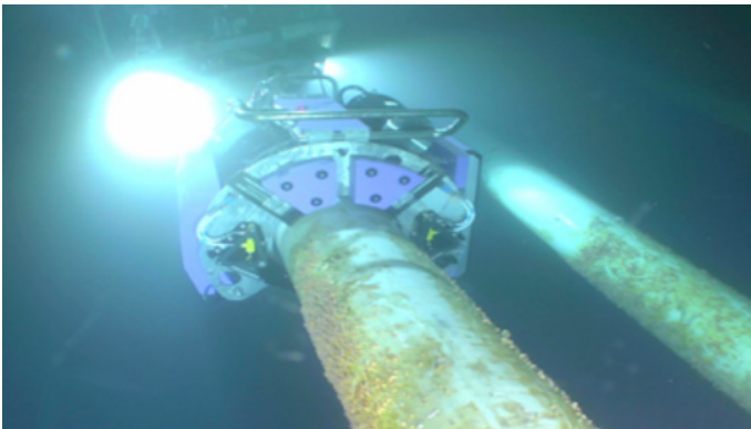
Figure 1: ARTEMIS scanning of shallow water flexible riser section in the North Sea.
