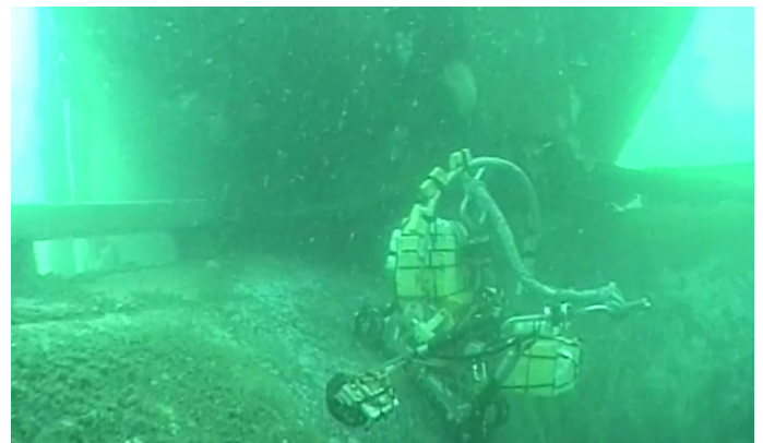
Figure 2: ACFM NodeScanner performing inspection underwater
