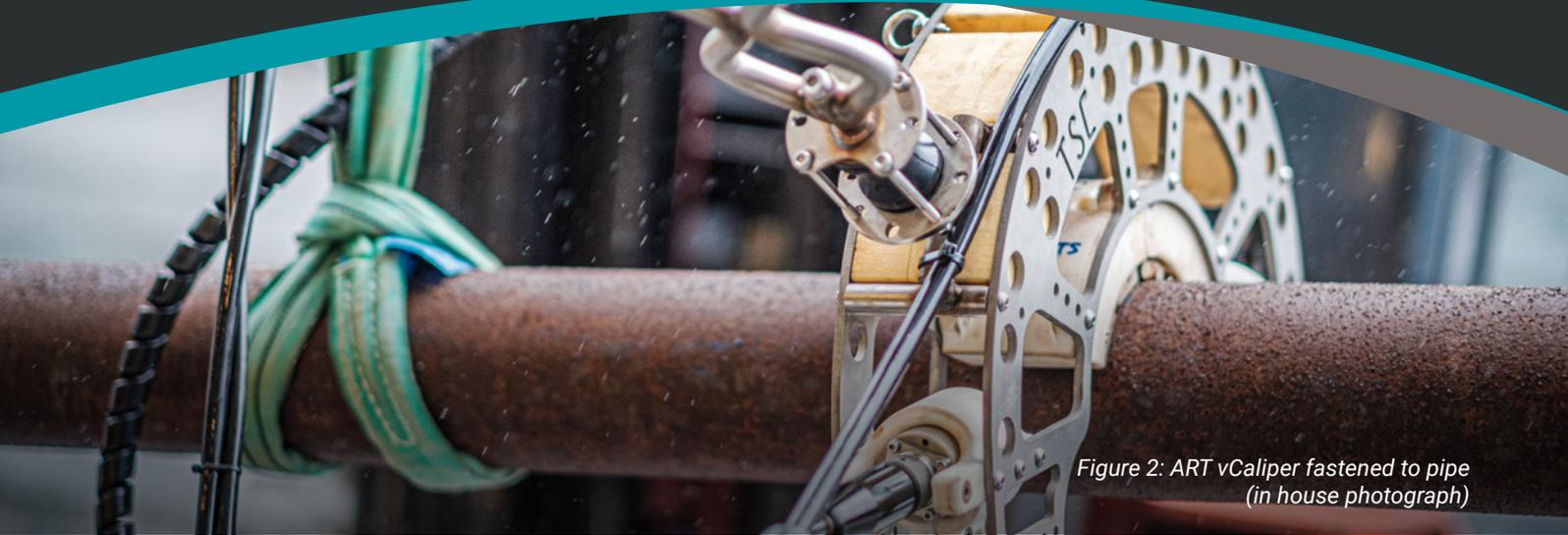
Figure 2: ART vCaliper fastened to pipe
